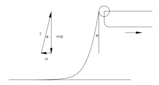
The total tension is the weight of cable + horizontal residual tension,
