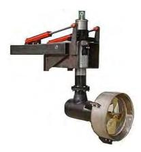
These thrusters can turn 360° and be leveled upwards when not in use. The most sophisticated steering system is when the thrusters are connected to a GPS system and linked to the route coordinates. (Dynamic Positioning System). In any case a GPS system is useful. It will monitor the position of laid cables.
