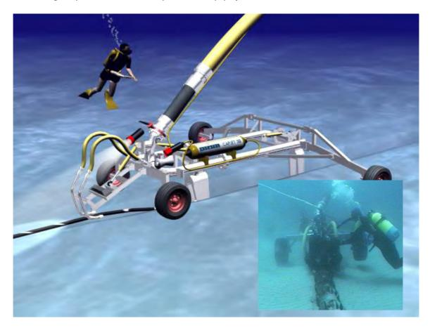
Figure 2 During 3m trenching in Gibraltar (3m)
