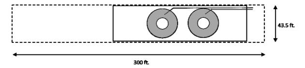
Barge inside a lock. The dotted line represents the lock dimension.
