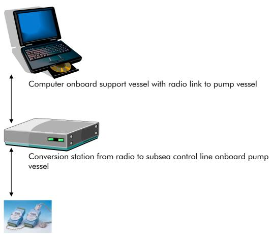
Subsea Control system on trencher (sensor, valves, light, thusters) OPC interface
