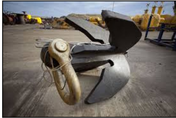
11 Figure 2-10. Example of Grapnel Used for Debris Removal
