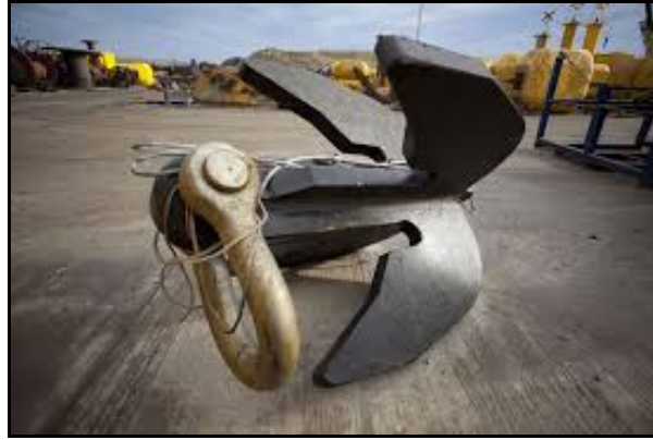
Figure 2-8. Example of Grapnel Used for Debris Removal
